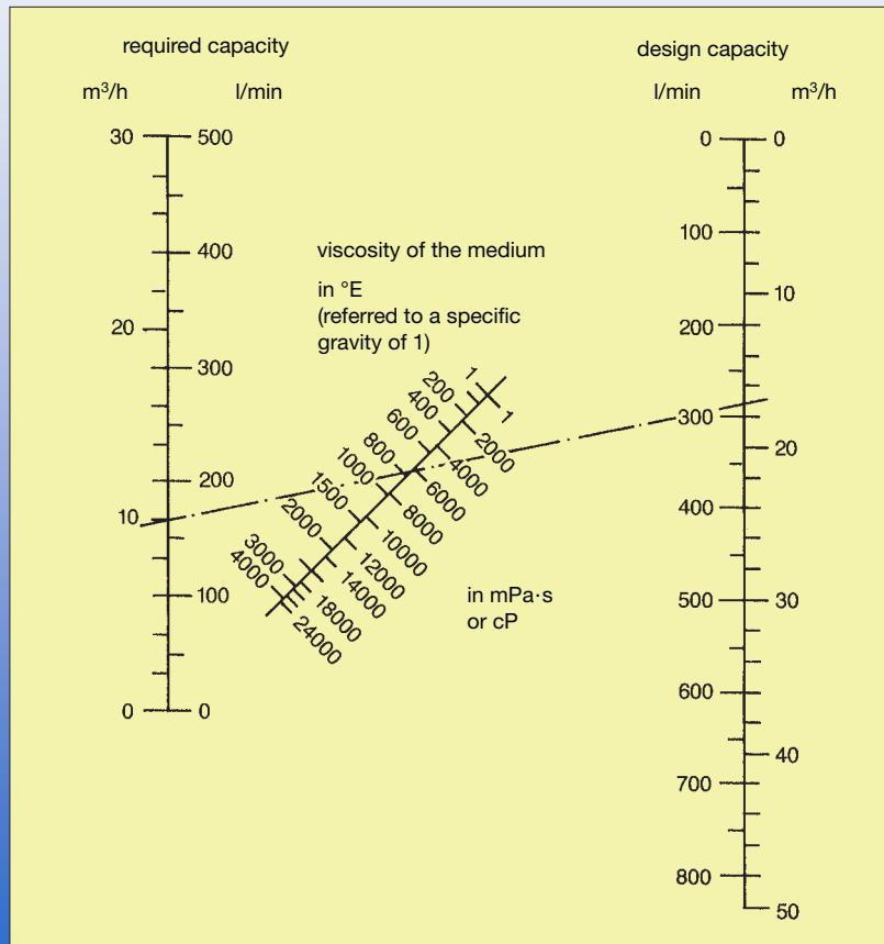
The capacity specified in the pump performance charts generally refer to water (1 mPas).
